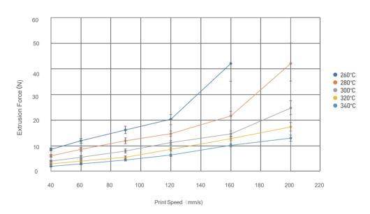
Test parameters: 12mm length brass heat block, BMG extruder, Hardened Steel Nozzle, Nozzle size 0.4mm, Layer Height 0.2mm.
